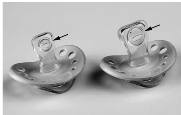
Fig. 2. The novel slow-release pacifier with pouch (↑).
